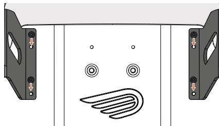
Figure 4 - Placing and attaching front bench.
