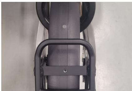
*Figure 8 - Drill hole in mudguard.*
