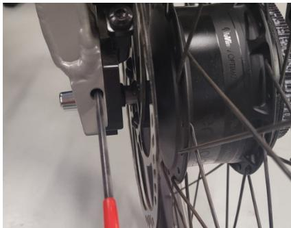
*Figure 3 - Remove tension from the belt.*
