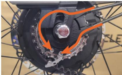
Figure 11 - Reposition gear cables.
