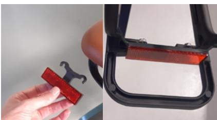
*Figure 1 - Mounting reflector on bike rack.*
