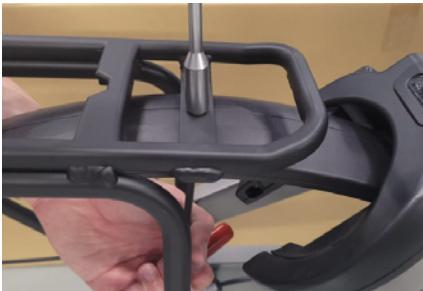
Figure 9 - Securing luggage carrier to fender.
