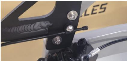
Figure 10 - Tighten luggage carrier and mudguard rods bolts.
