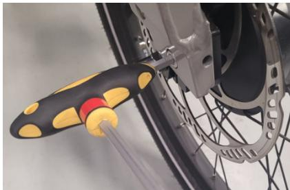
Figure 13 - Securing dropouts.
