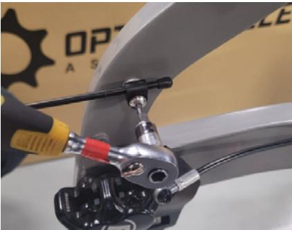
*Figure 5 - Removing the mudguard rods.*
