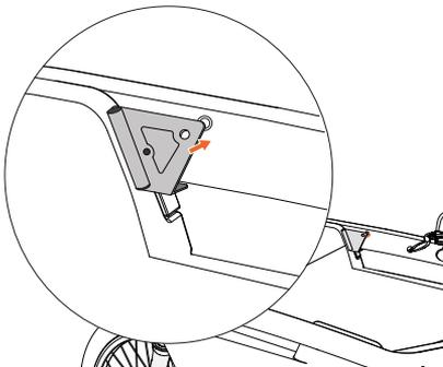
Figure 4 - Attaching the adapters to the frame.
