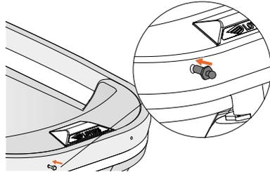
Figure 5 - Attaching the screw with press connector.
