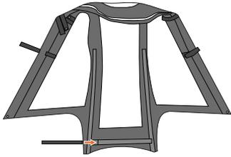
Figure 2 - Placing connecting rod in rain cover.
