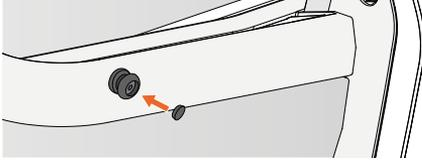
Figure 8 - Closing loop connectors.
