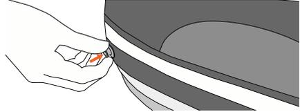
Figure 11 - Attaching press connectors front side.
