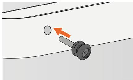
Figure 7 - Attaching the screw with loop connector.
