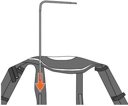
Figure 3 - Placing rod assembly in rain cover.
